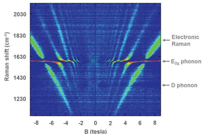
**Figure 5:** Micro-Raman spectra of a graphene flake as function of the magnetic field. The spectrum at  $B=0\text{ T}$  has been subtracted.
