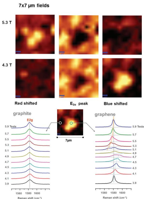
**Figure 4:** Raman mapping of a graphene flake on graphite. The magnetic field values ( $B=4.3\text{ T}$  and  $B=5.3\text{ T}$ ) are chosen to be just below and just above the resonant condition for electron-phonon hybridization.
