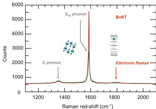
**Figure 3:** Raman spectra of graphene acquired at 7 K and at  $B=0\text{ T}$  (red) and  $B=9\text{ T}$  (green) showing a magnetic field dependent band at  $1800\text{ cm}^{-1}$ .
